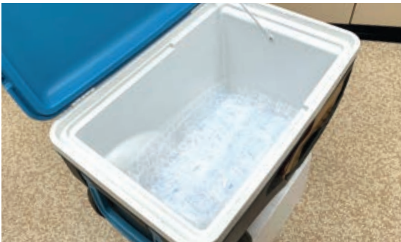
Figure 3: Insulating material placed in bottom of cooler
